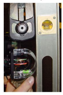
Some sights feature 2nd and 3rd axis adjustments options. Admittedly, these features probably aren't necessary for a general purpose hunting rig. But for us hard-core enthusiasts and pathological tinkerers, these advanced adjustments are handy innovations. 2nd & 3rd Axis adjustments essentially ensure that your sight's bubble level is always telling you the truth.
