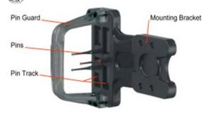
Some bow sights are quite simple, like the one on the left. This is an example of a straightforward fibre-optic 3-pin composite (plastic) sight, with a Lexan pin guard, and twin pin tracks. Each pin can be positioned up or down in its track for elevation adjustments and each pin can be screwed in and out of the mounting bracket for windage adjustments.
