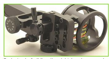
Generally, gang adjustments are made by loosening a screw and then sliding the sight housing to a new position. But some sights are designed with a micro-adjust feature which allows gang windage and elevation adjustments to be made by turning an adjustment knob (usually attached to a simple gear that drives the motion of the housing).
